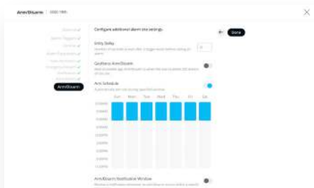
7 Virtual Guard is only enabled when the designated site is "Armed." You can manually arm and disarm the site via Command, or set an Arm schedule. Site should only be armed after hours or during periods where human activity in the selected cameras/regions is unexpected and represents a potential threat to people or property.
