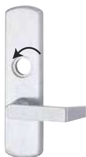
Key retracts latch bolt. Lever or knob is rigid. Use NL suffix, e.g., 996LNL. (Storeroom)
